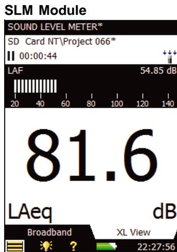
2250 Light comes with the Sound Level Meter Software for 2250 Light included. This makes 2250 Light into a versatile broadband sound level meter; it complies with the latest international standard (IEC 61672-1) as well as previous international and national standards.
