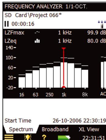
1/1-octave Frequency Analysis Software for 2250 Light BZ-7131, and 1/3-octave Frequency Analysis Software for 2250 Light BZ-7132 are optional software modules. They allow you to make real-time measurements in 1/1- or 1/3-octave bands over a wide frequency range. This makes it a simple matter to obtain spectra in order to, for example, select hearing protection, qualify heat and ventilation systems, and assess tonality.
