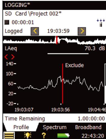
With the optional Logging Software enabled, 2250 Light becomes a versatile instrument for obtaining time histories. The Logging Software allows you to select freely among the broadband parameters and log them at intervals from 1 s to 24 h. At the same time  $L_{Aeq}$  and/or  $L_{AF}$  can be logged at 100 ms intervals.
